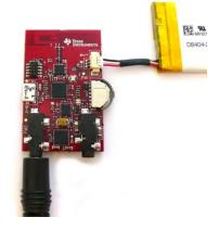
Connect an audio source (CD-player, MP3-player or similar) to the line in connector on the Master Headset board (labeled Master on the back side) via the 3.5mm jack cable.
