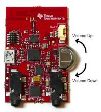
The pre-programmed Slave firmware is configured to have so-called "local volume control" meaning that the Slave controls its own volume locally. The volume buttons are mapped to clicking/holding the rocker switch UP and DOWN.
