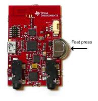
In the pre-programmed firmware the pairing button is mapped to pressing the rocker switch IN (not hold, which is power toggling as described in 4).
