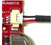
There's only one way to connect the battery plug to the socket on the board. With the pre-programmed firmware the CC8531 enters the OFF power mode when the battery is connected. The batteries should have enough charge out-of-the-box to establish a link and stream audio. To charge the battery, see section 9. With full battery the link should run for typically 15 hours, the Master being the bottleneck. The Slave plays audio for 22 hours typically.
