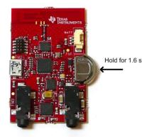
In the pre-programmed firmware the toggling between power modes OFF and ON is mapped to pressing the rocker switch IN for 1.6 seconds. The two boards are unpaired out-of-the-box, so in the ON power mode the topmost LED should flash once every second indicating network state ALONE . In the OFF power mode the LED is turned off. Make sure both boards are flashing.
