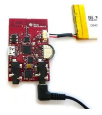
Connect a headphone to the 3.5mm headphone output on the board labeled Slave on the back side.
