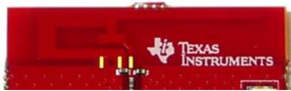
Figure 2 CC85xxHeadset PCB antenna
