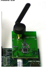
Connect the CC85xxEM or the CC85xx-CC2590EM marked MASTER (label attached on the backside of the board). These boards are pre-programmed with master firmware. Attach the antenna to the SMA connector.
