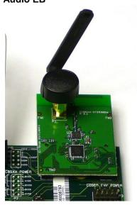
Connect the CC85xxEM or the CC85xx-CC2590EM marked SLAVE (label attached on the backside of the board.) These boards are pre-programmed with slave firmware. Attach the antenna to the SMA connector.
