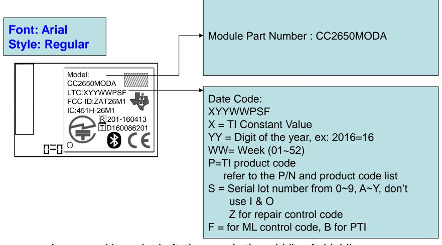
Laser marking rule draft, the area in the middle of shielding case
