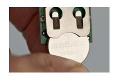
Note that when inserting the battery for the first time, the PCB contact point surface has a thin layer of solder residue that may prevent contact with the battery. Remove and insert the battery a few times to power the SensorTag.
