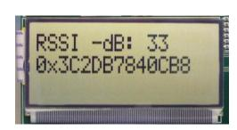
If the boards are moved farther apart from each other, the RSSI will drop (since the value is negative, a higher number means lower RSSI). If they are moved closer together, the RSSI should
