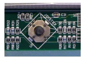
The joystick has five different movements: it can be moved up, down, left, right, and it can be pressed in, just like a button. Each movement performs different actions depending on the state of the device.
