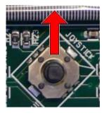
After a few seconds, it should display "Devices Found 1 / <- To Select". This means that the central device successfully discovered the peripheral. Press left on joystick U1 to view the address of the peripheral device. This address should match the address seen on the peripheral's LCD.
