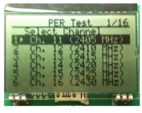
Select which channel to use for the test.
