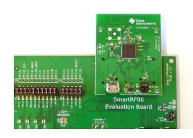
Insert a CC2538EM board into the SmartRF06EB as shown above.
