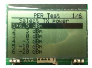
On the transmitter, select desired output power.
