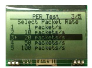
On the transmitter, select the desired packet
