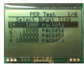
On the transmitter, select the desired burst size, that is, the number of packets to transmit.
