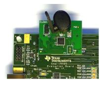
The CC2530EM, with the antenna mounted on the SMA connector, can be plugged into a SmartRF05EB. The SmartRF05EB is included in the CC2530 Development Kit [2].
