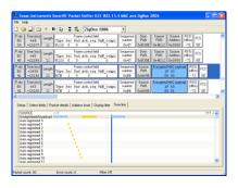
You can use the CC2531 USB dongle or the SmartRF05EB with a CC2530EM to capture the packets.
