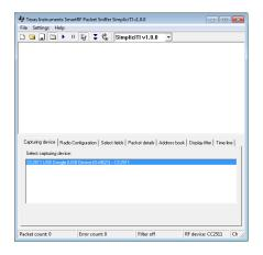
The USB dongle should be listed with chip type CC2511 and EB type CC2511 USB dongle in the "Capturing Device" tab.
