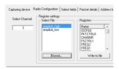
If this is the first time you use the tool, press the browse button to locate a .prs file with packet sniffer register settings for CC2511.
