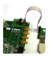
**Caution!** Avoid using other power sources<sup>1</sup> for the dongle than a regular USB voltage source at max 5.5V, 500 mA, (efficiency level V).
