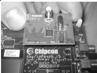
Insert a CC2510EM into both SmartRF04EBs. Make sure the antenna is firmly connected to the SMA connector.
