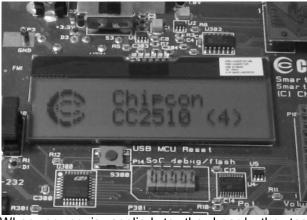
When power is applied to the board, the test program will start. You should see the Chipcon logo with chip name and revision number as shown above on the LCD display on both EBs. Pushing button S1 in the lower right corner of the board will show the first menu item.
