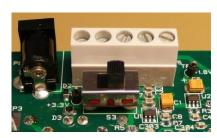
If a 3.3V source is used as described in 4b above, the switch should be set to the leftmost position. For all other cases, the switch should be set to the rightmost position. This switch can be used to turn off the EB by switching it to the opposite position of that used to turn it on
