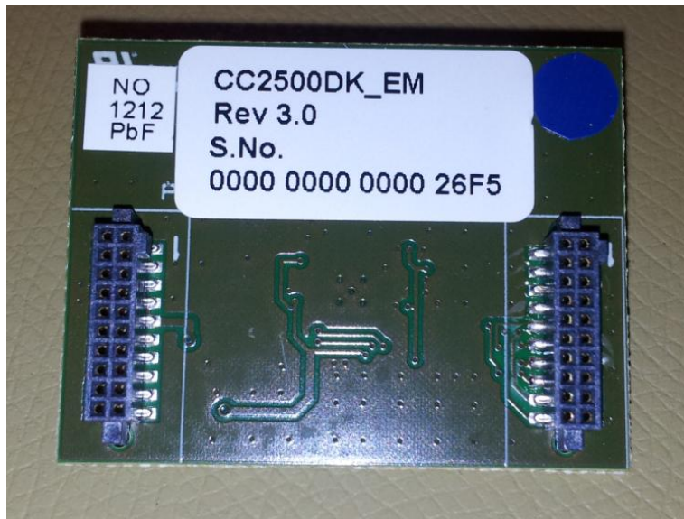
Figure 2 - CC2500EM Rev 3.0 - Bottom view
