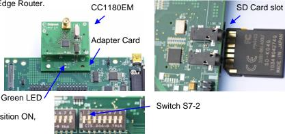
It will take approximately 40 seconds to boot the Edge Router. When the green LED on the Adapter Card goes ON it indicates that the Edge Router is up and running. You can connect the provided RS-232 NULL modem cable between the Edge Router and PC to get debug information, use e.g. Windows HyperTerminal with settings; Baud Rate 115200, 8 Data Bits, No Parity, One Stop Bit and No Flow Control.
