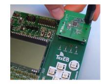
Insert the CC1175EM into a TrxEB as shown above. Do not use excessive force on the EM. Remember to mount the antenna.
