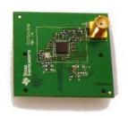
1 x CC1175 Evaluation Module 868/915 MHz 1 x Pulse W5017 Antenna (2 dBi gain)
