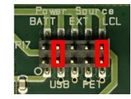
Depending on the power source, make sure you connect jumpers to the appropriate pins on the "Power Source" header. For instance, if you use batteries, use a jumper to short-circuit pin 1 and 2 on the header. The last jumper in the row (pin 9-10) should always be mounted, unless the MSP430 FET is used as the power source.
