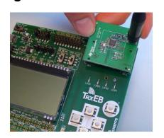
Insert a CC112xEM into the TrxEB. Do not use excessive force on the EM. Remember to mount the antenna.
