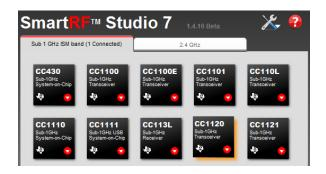
After installing the tool, connect the EB to the PC using the USB cable and start SmartRF Studio. Select the "Sub 1 GHz" tab and double click the highlighted CC1120 or CC1121 device icon.
