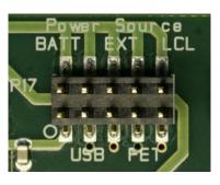
Depending on the power source, make sure you connect jumpers to the appropriate pins on the "Power Source" header. For instance, if you use batteries, use a jumper to short-circuit pin 1 and 2 on the header. See back side of board for explanation of the jumpers.
