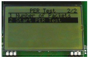
When selecting "Start PER Test", the master Press the "Up" button to go to the detailed (receiver) will begin to count the number of received packets and provide some statistics.
