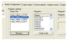
If this is the first time you use the tool, press the browse button to locate a .prs file with packet sniffer register settings for CC1111.
