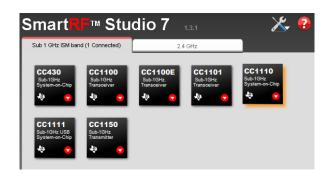
After installing the tool, connect the EB to the PC using the USB cable and start SmartRF Studio. Select the "Sub 1 GHz" tab and double click the CC1110 device icon.
