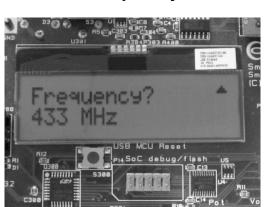
Select the frequency that you want to use (433 MHz, 868 MHz, 903 MHz or 915 MHz). Move the joystick up or down to display the choices and push button S1 in the lower right corner of the board to select the displayed frequency.
