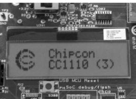
When power is applied to the board, the test program will start. You should see the Chipcon logo with chip name and revision number as shown above on the LCD display on both EBs. Pushing button S1 in the lower right corner of the board will show the first menu item.
