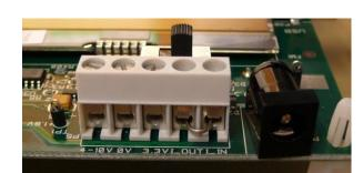
The second method applies DC power using the DC input jack (right in picture, centre is +, sleeve is ground), or by connecting a 4-10V voltage source between the 4-10V and 0V terminals of the power connector (left in picture). It is also possible to connect a 3.3V voltage source between the 3.3V and 0V terminals. The on-board voltage regulators will be bypassed in this case.
