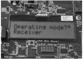
Select Receiver on the first EB by moving the joystick. Confirm by pressing button S1. The Receiving node will display "Ready to receive".
