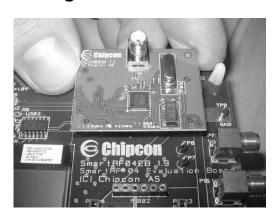
Insert a CC1110EM into both SmartRF04EBs. The connectors will only fit in one position, so that the EM cannot be inserted the wrong way. Do not force the EM. Remember to connect the antenna as well.
