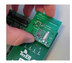
Insert a CC110LEM into the TrxEB. Do not use excessive force on the EM.
