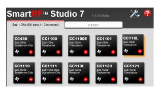
using the USB cable and start SmartRF Studio. settings and run performance tests of the radio. Select the "Sub 1 GHz" tab and double click the highlighted device icon (CC110L, CC113L or CC115L).
