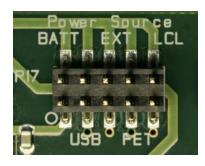
connect jumpers to the appropriate pins on the "Power Source" header. For instance, if you use batteries, use a jumper to short-circuit pin 1 and 2 on the header. The last jumper in the row (pin 9-10) should always be mounted, unless the MSP430 FET is used as the power source.
