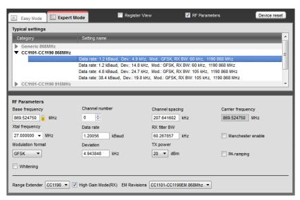
In order to control the CC1190 select CC1190 as "Range Extender" and select the appropriate "EM Revisions" as shown (either 869 or 915 MHz). You can now use all the features in Studio as for a standalone EM. Test the performance of the radio using some of these features:
