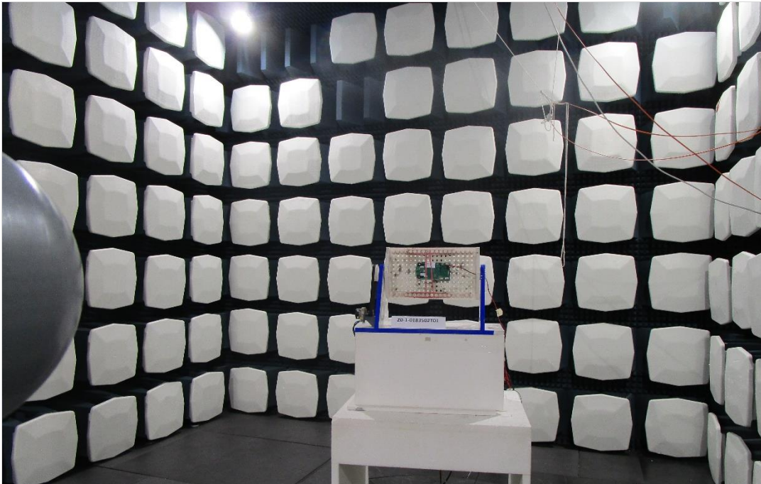
Photograph 5: EUT Test Setup in the fully anechoic chamber, Radiated interference field strength
