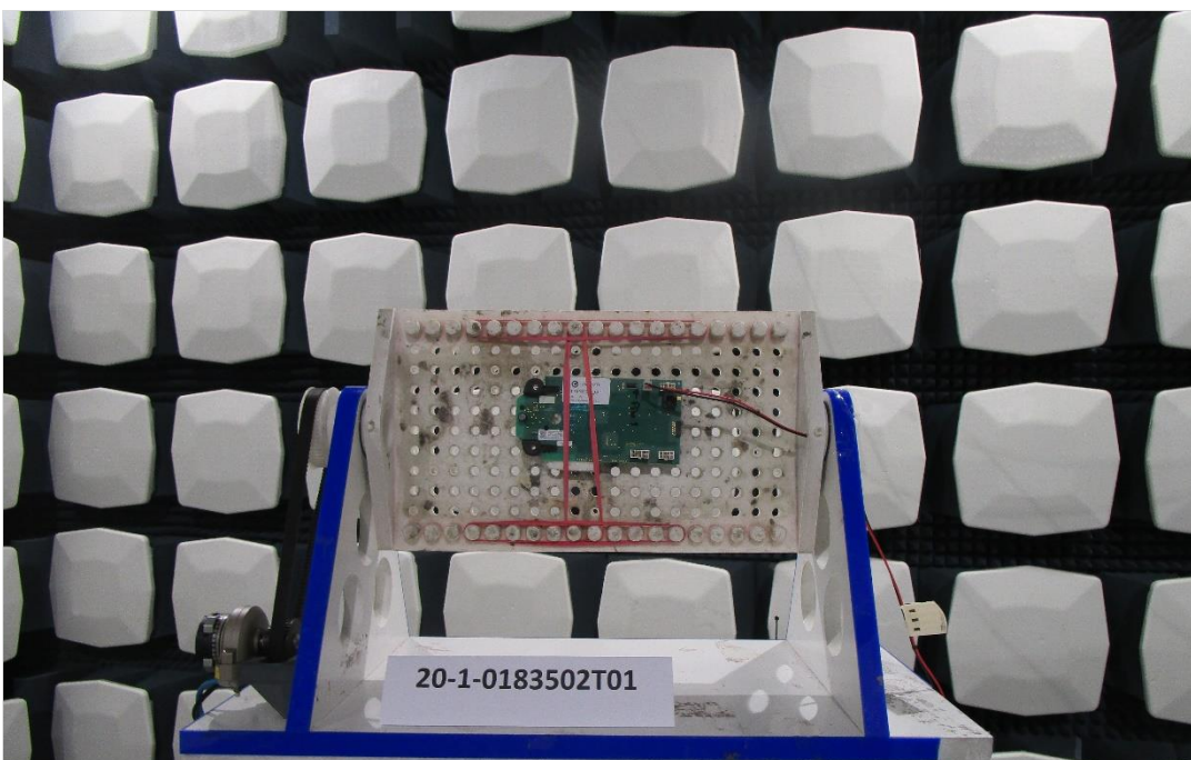
Photograph 6: EUT Test Setup in the fully anechoic chamber, Radiated interference field strength
