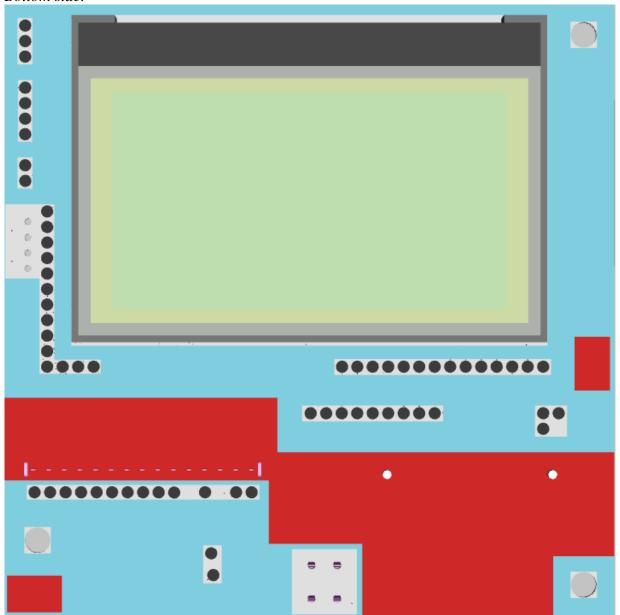
The whole viewing area of the display shall be masked during display side coating. Make sure that coating residuals do not cover the edge of the display.
