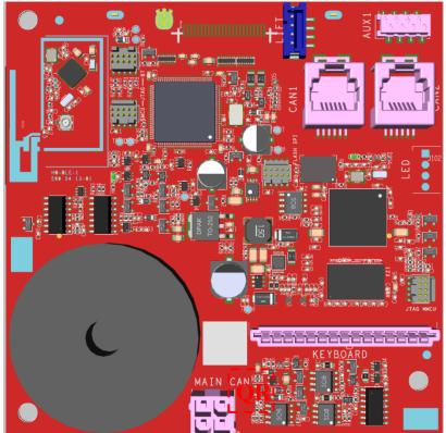
Manufacturer specific QR-code can be added in above square on top side, as seen above. (If the manufacturer of the PCB wishes to place his logo on the PCBA, this could be placed in the solder mask or on a label. It must not be placed in the copper layer.)
