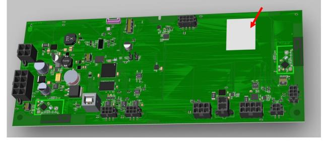
(If the manufacturer of the PCB wishes to place his logo on the PCBA, this could be placed in the solder mask or on a label. It must not be placed in the copper layer.)
