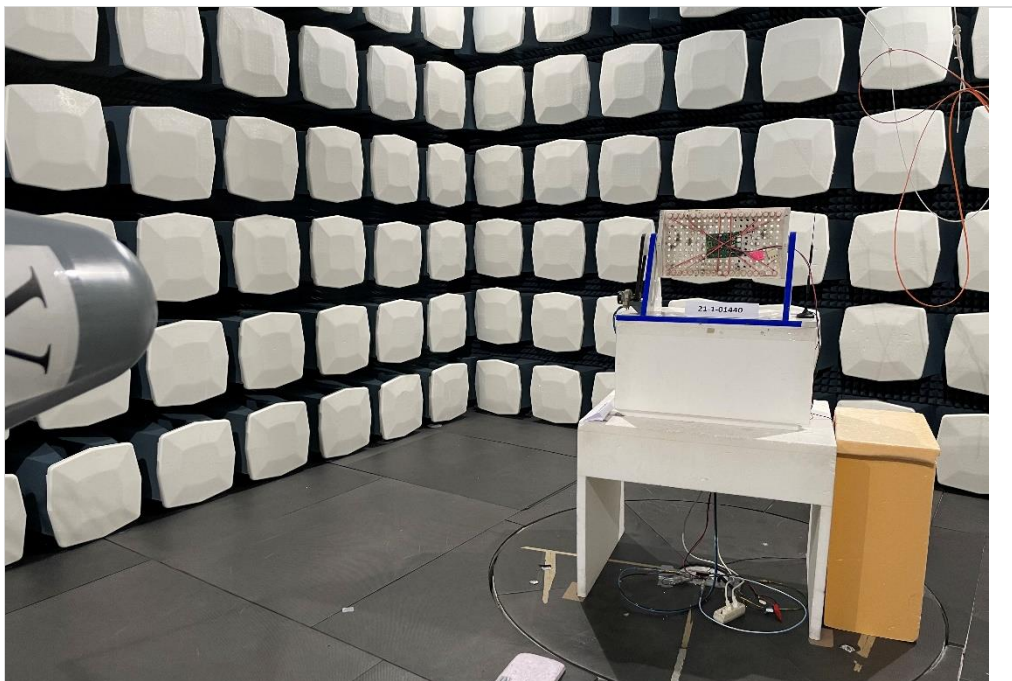
Photograph 2: EUT test setup in the fully anechoic chamber, overview
