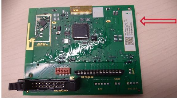
PCB 582 87 12, used in HMI Board Type 10, HMI Board Type 11 and HMI Board Type 12
