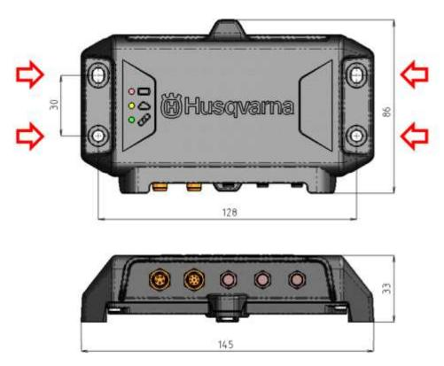
Fastening using 4 pcs, M5 bolts and washer
