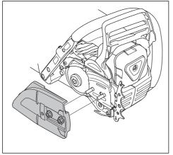
**Note:** If the clutch cover is not easy to remove, tighten the bar nut, engage the chain brake and release. A click is heard if it is released correctly.
