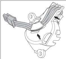
4. Put the holder for the Husqvarna connectivity device on the air filter holder and install the 2 screws.
