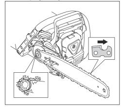
6. Align the hole in the guide bar with the chain adjuster pin and install the clutch cover.
