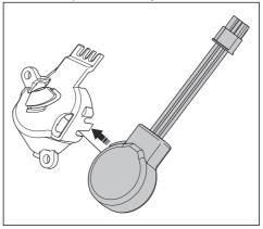
3. Attach the wires to the holder for the Husqvarna connectivity device.
