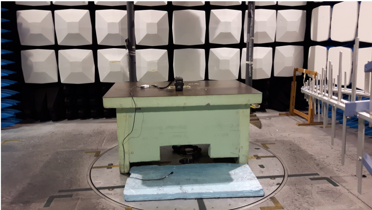
Test set up radiated emission 30 MHz – 1GHz
