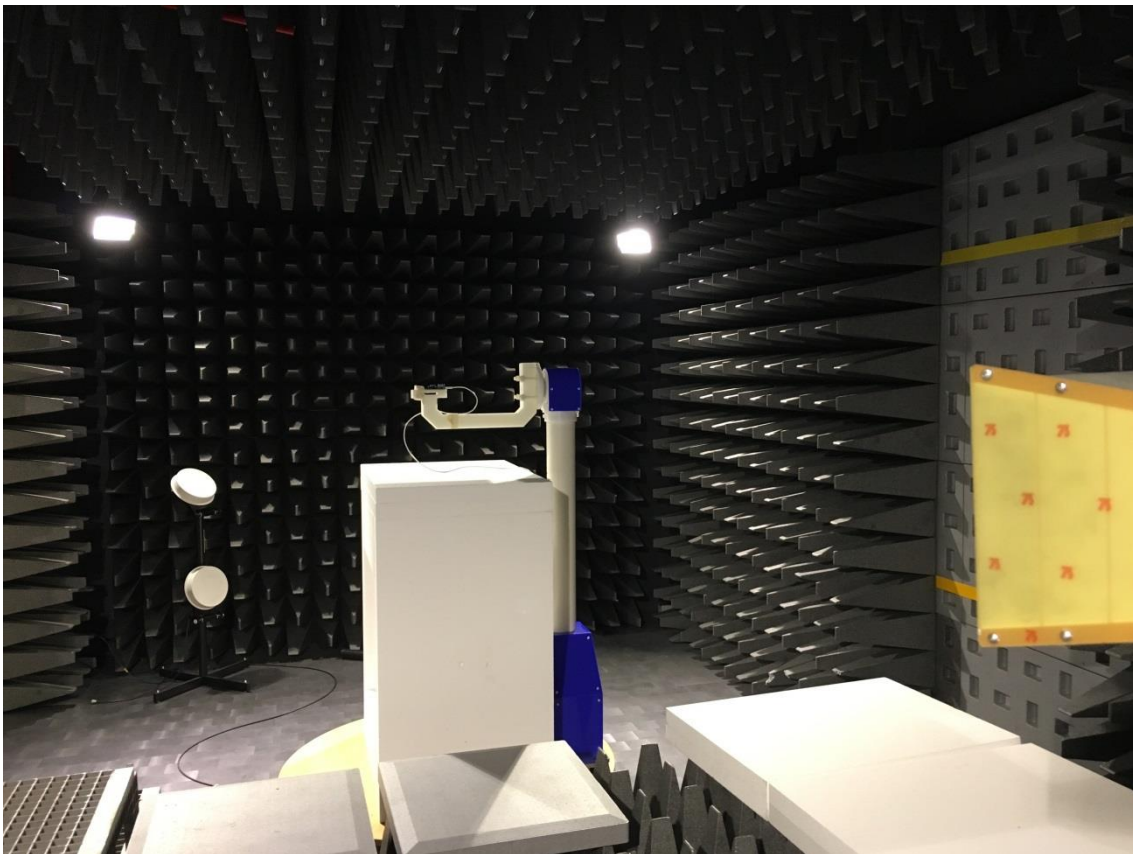
Test set up radiated emission above 1 GHz
