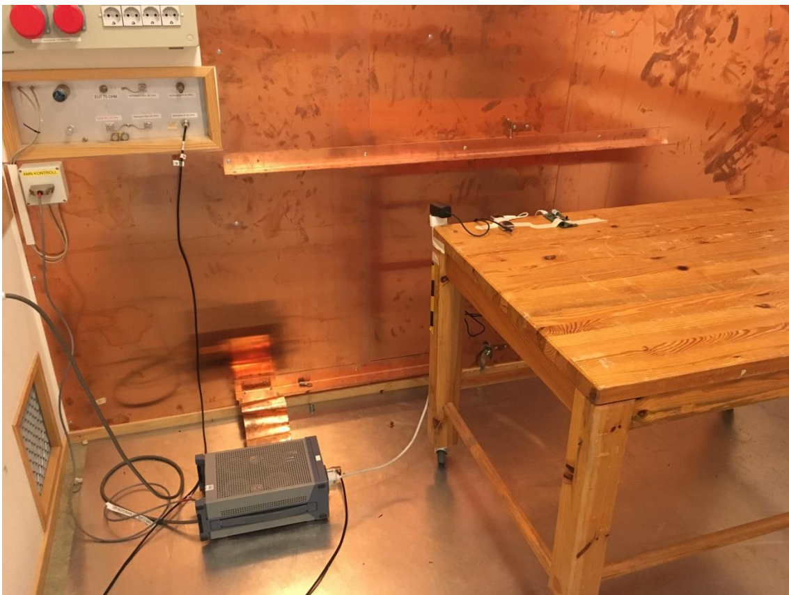
Test set up conducted emission 9 kHz – 30 MHz
