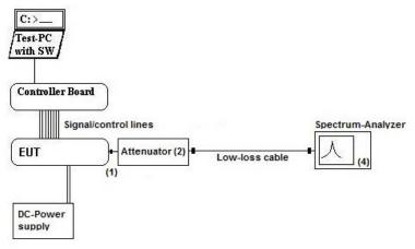
**Testing method:** ANSI C63.10:2013, KDB 558074 D01 DTS Meas.Guidance v03r02
