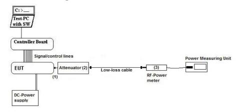
**Testing method:** ANSI C63.10:2013, KDB 558074 D01 DTS Meas.Guidance v03r05
