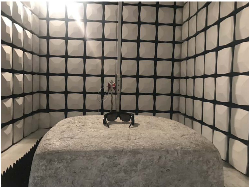
Description: Radiated Emission Test Setup for 1~18GHz
