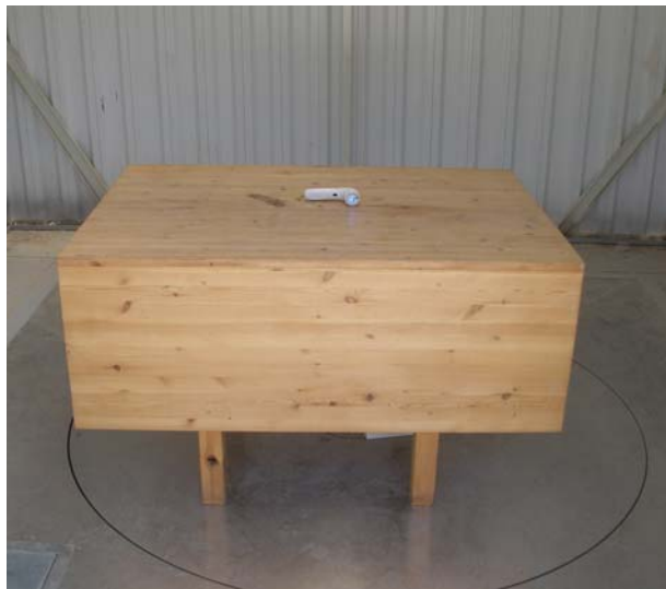
Photo 4. RE test setup on OATS.
