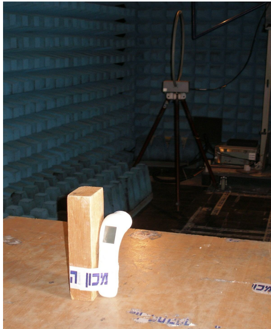
RE test setup in anechoic chamber.
