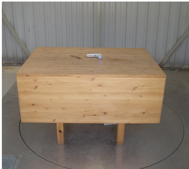
RE test setup on OATS.
