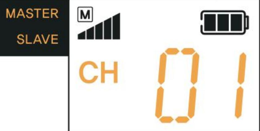
1. If you press the MENU button, the [CH] icon will blink. In this case, change channels by using ▲ (UP)/ ▼ (Down) button.
