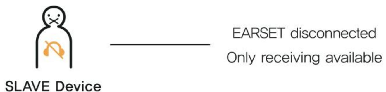
The MASTER device has the same function of having / cancelling the right to speak as the SLAVE device. However, if the EARSET is disconnected from the SLAVE device, the receiving function of the SLAVE device is only available without having the right to speak.
