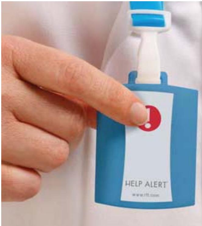
When the alarm is acknowledged at the monitoring station, the light now flashes green in 10-second intervals to indicate that the alarm is now in an acknowledged state. Clearing the alarm at the monitoring station automatically resets the Pendant for the next distress call.
