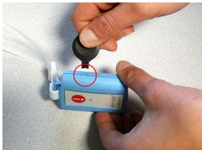
2. If changing the batteries, use a small, non-conductive piece of plastic or wood to pop the battery free from the battery holder.
