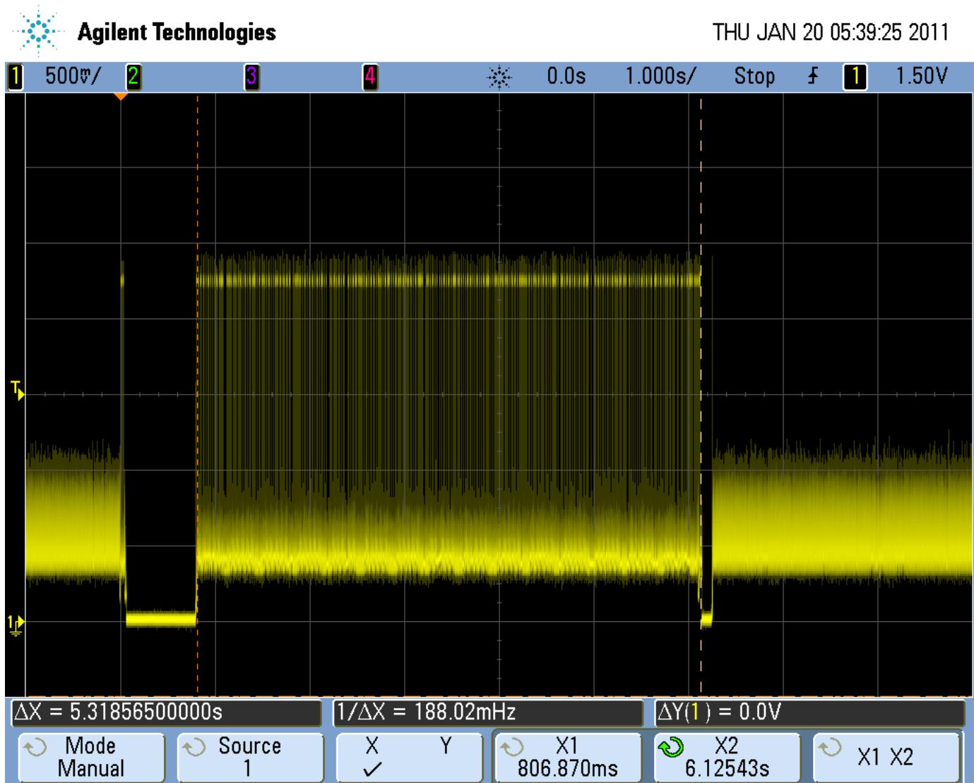
As can be seen, the communication phase has increased to 5.319 seconds due to the repetitive scanning for an Access Point.
