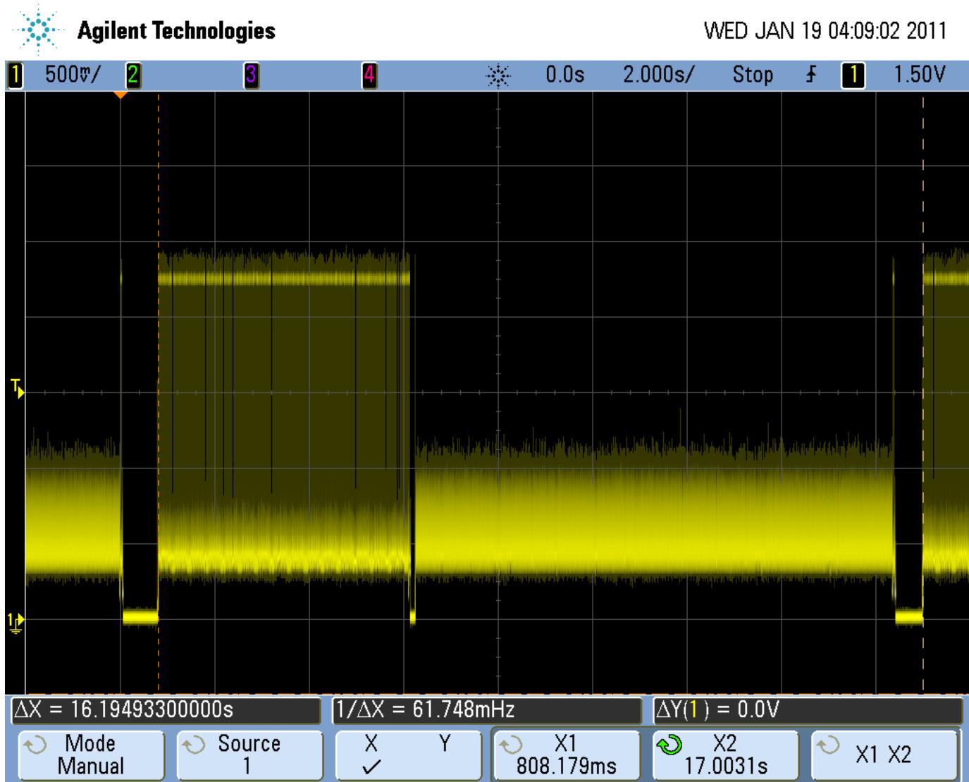
As can be seen, the overall period of one alarm cycle in this case is 16.195 seconds.
