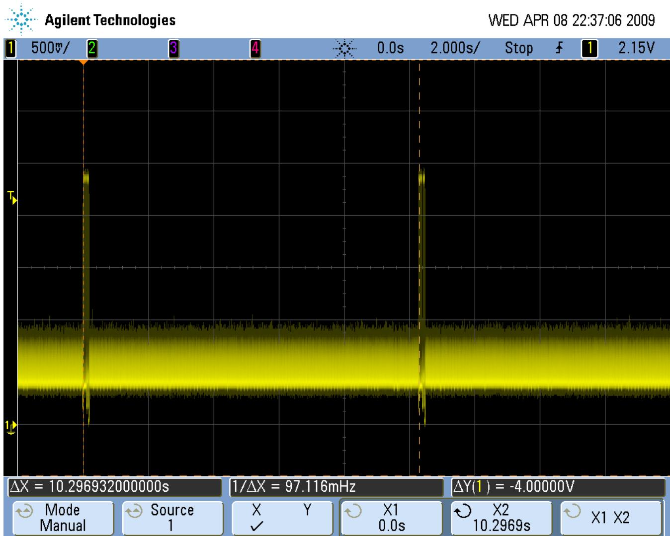
In this case, the communication phase consists of the activity at the beginning denoted by the red marker on the left. The listening phase consists of the region after the communication phase and terminated where denoted by the red marker on the
