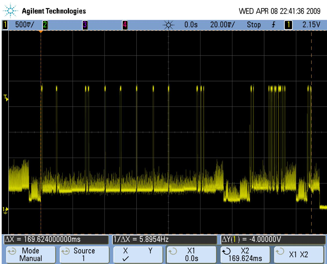
As can be seen, there is a variety of transmit activity that occurs during this phase. In particular, starting at the left are the probe requests that are sent while active scanning is performed. Once the AP is located, typical WiFi and other networking protocols are followed before the UDP packet is finally sent. In addition, at the very end of this phase, the Tag also sends the UDP packet to a PDA that is operating on an ad-hoc network.
