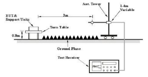
The radiated emission were performed in the 3 meters, using the setup accordance with the ANSI C63.4-2014. The specification used was the FCC Part 15.109 and ICES-003 Class B limits.
