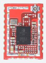
RED bean is a high performance and ultra low power surface mount SDIO radio combining single-stream 11ac Wave2 Wi-Fi and Bluetooth® 5.0 in a very small form factor
