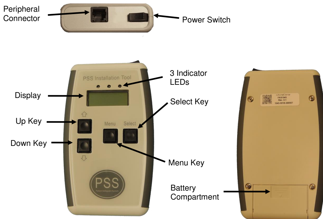
Figure 1 - FAS1543 Beacon Installation Tool's Features
