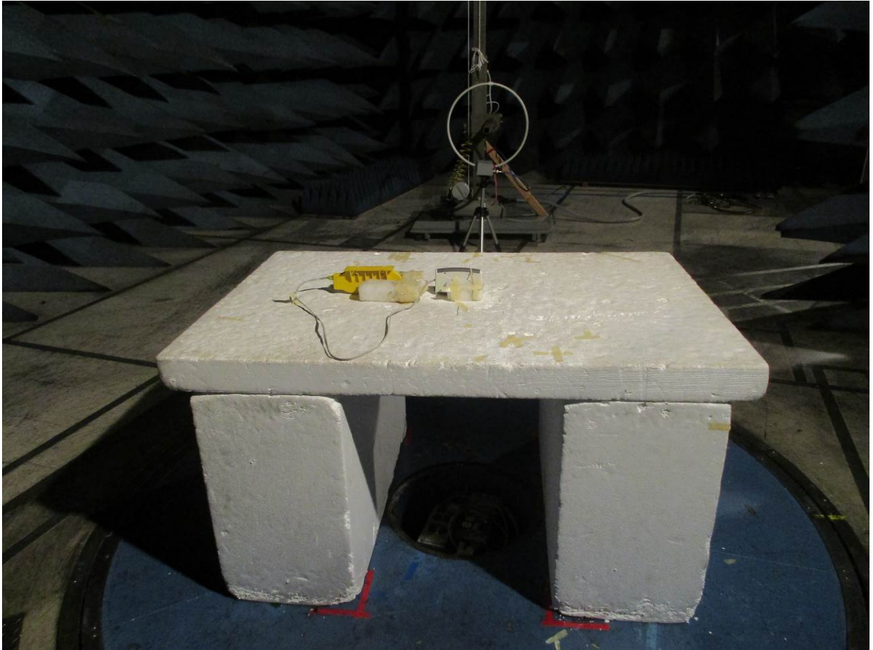
Figure 20: Radiated Emissions – Back View – 9 kHz – 30 MHz (125 kHz additional photos)
