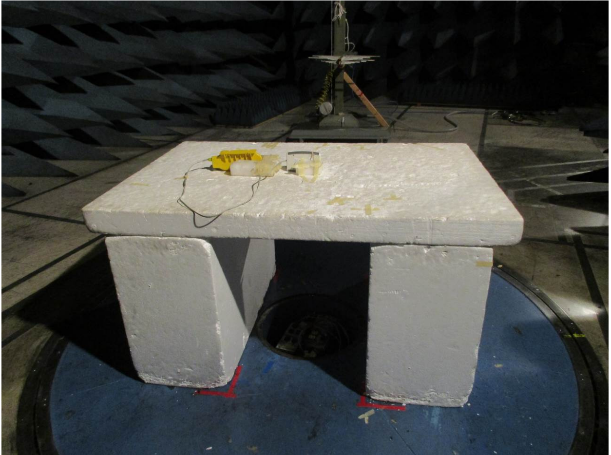
Figure 22: Radiated Emissions – Back View – 200 MHz – 1 GHz (125 kHz additional photos)
