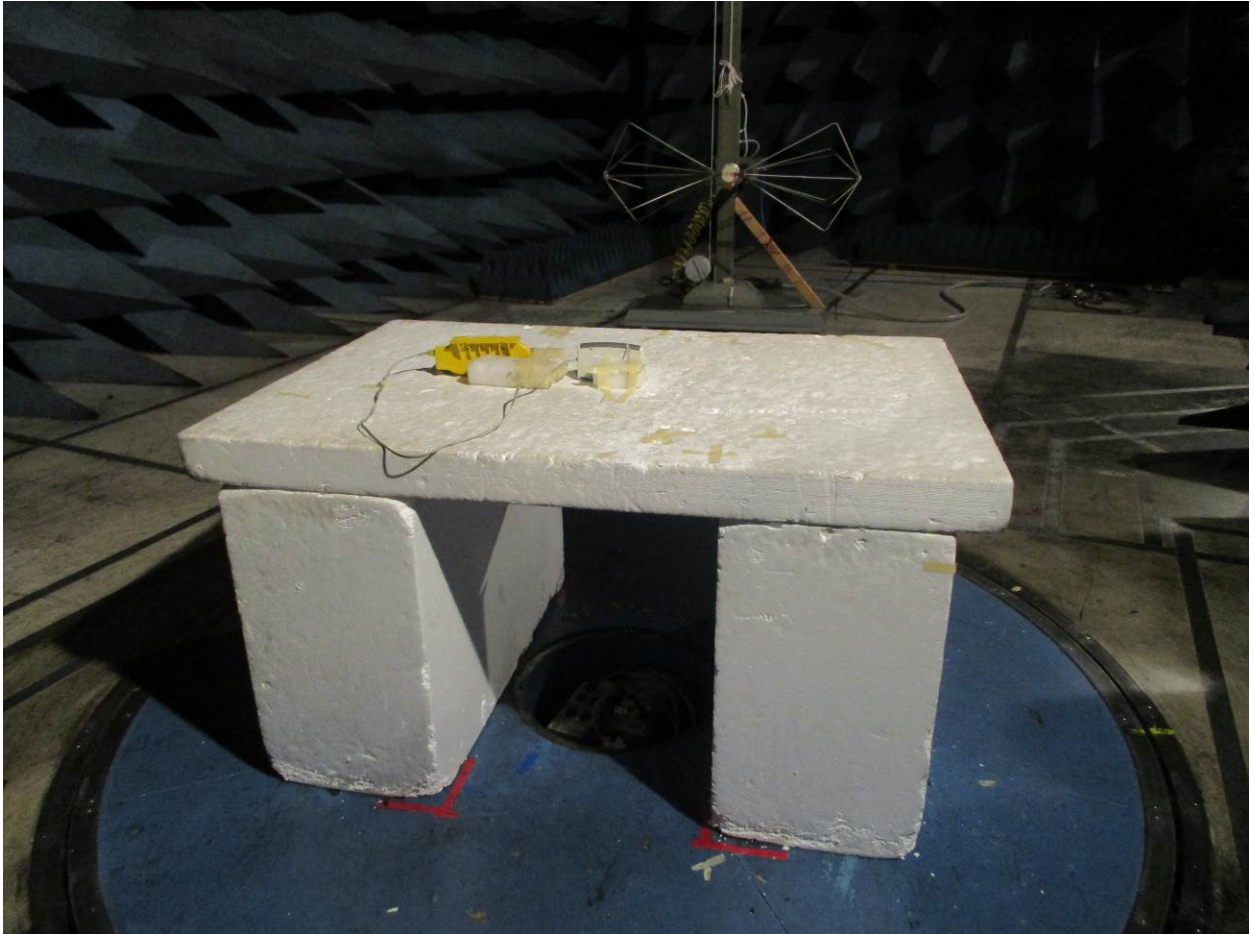
Figure 21: Radiated Emissions – Back View – 30 MHz – 200 MHz (125 kHz additional photos)
