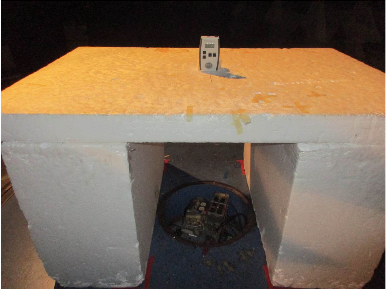
Figure 1: Radiated Emissions – Front View – Below 1 GHz (EUT Standing)
