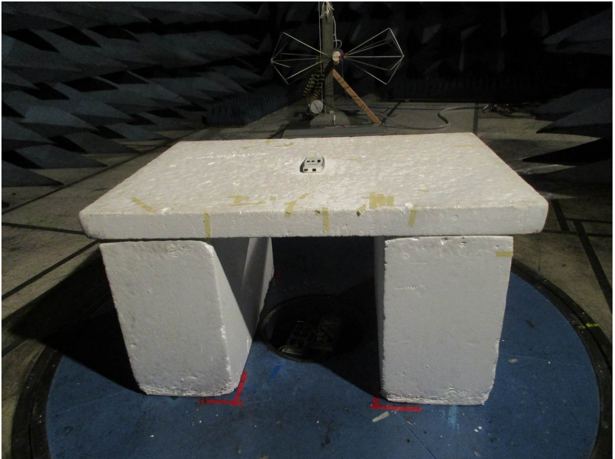
Figure 15: Radiated Emissions – Back View – 30 MHz – 200 MHz (EUT Flat)
