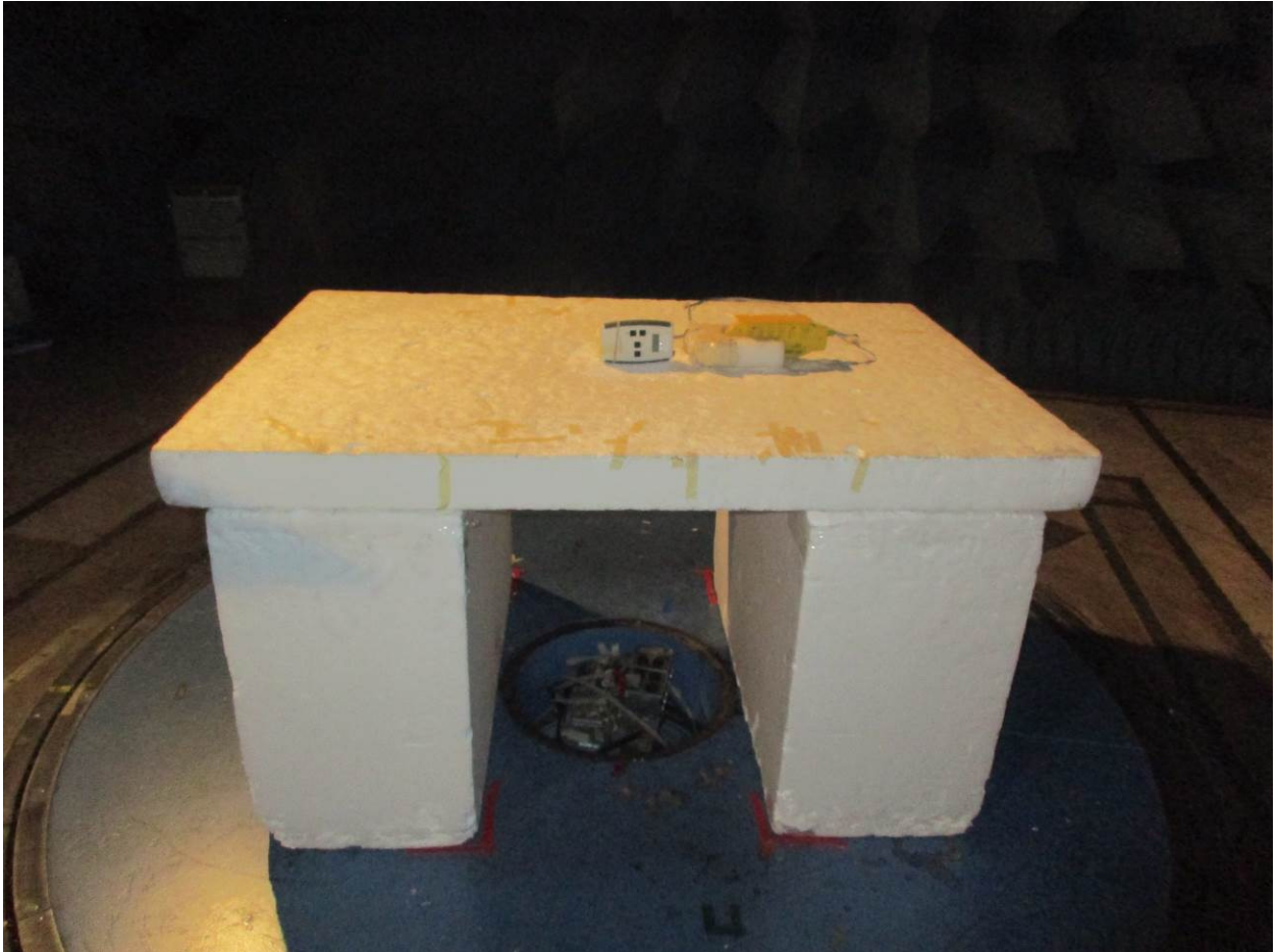
Figure 19: Radiated Emissions – Front View – Below 1 GHz (125 kHz additional photos)
