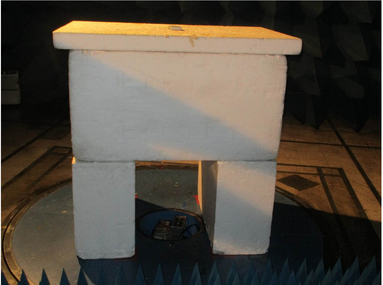
Figure 17: Radiated Emissions – Front View – Above 1 GHz (EUT Flat)
