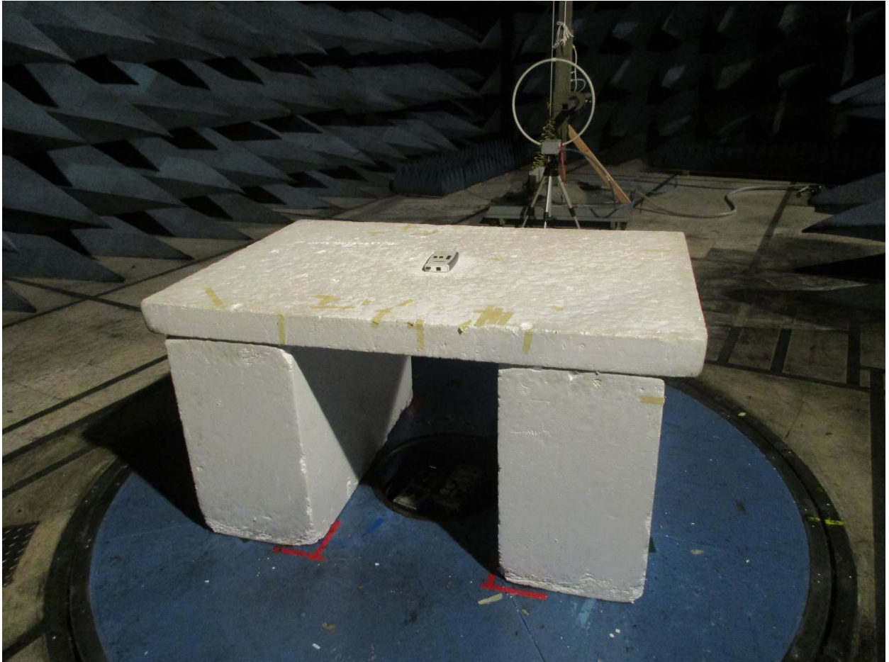
Figure 14: Radiated Emissions – Back View – 9 kHz – 30 MHz (EUT Flat)
