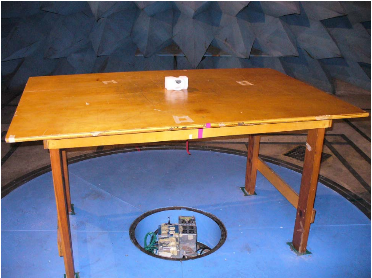
Figure 2: Radiated Emissions – Front View (XZ – Standing)
