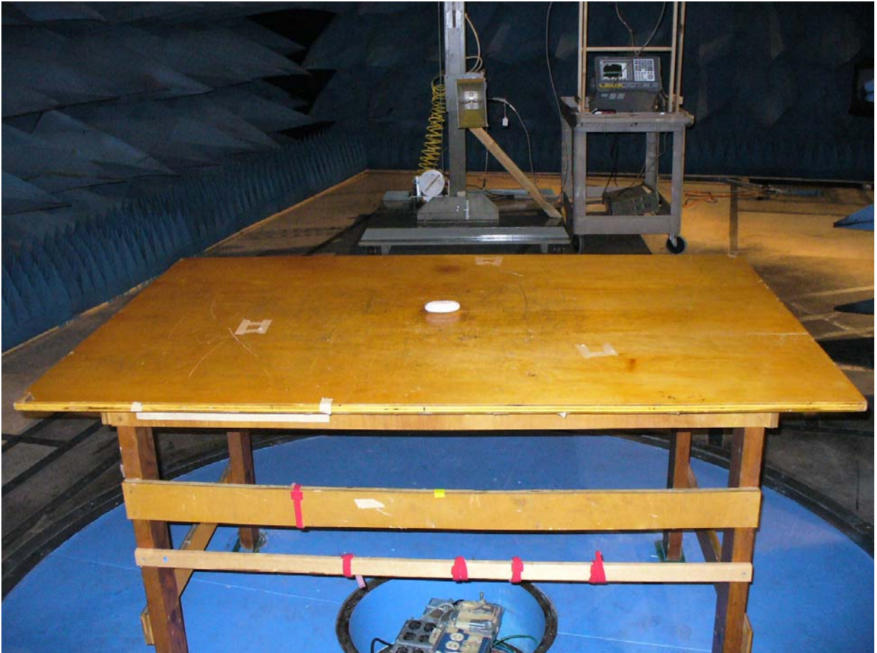
Figure 6: Radiated Emissions – Rear View (YZ – Flat)
