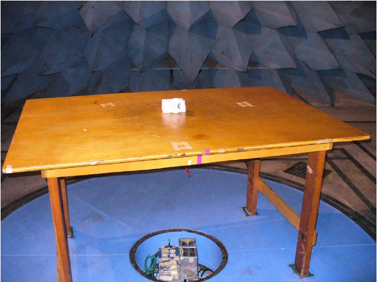
Figure 1: Radiated Emissions – Front View (XY – Side)
