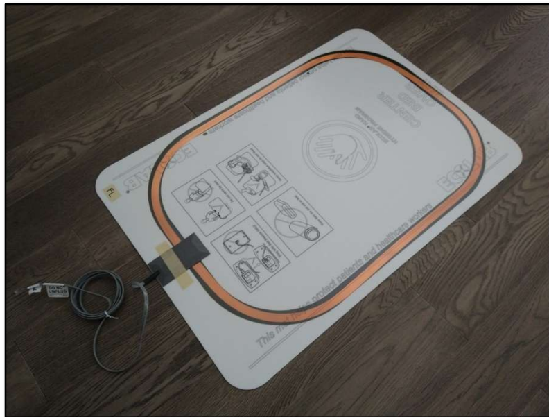
Figure 3. Production prototype flat spiral coil antenna
