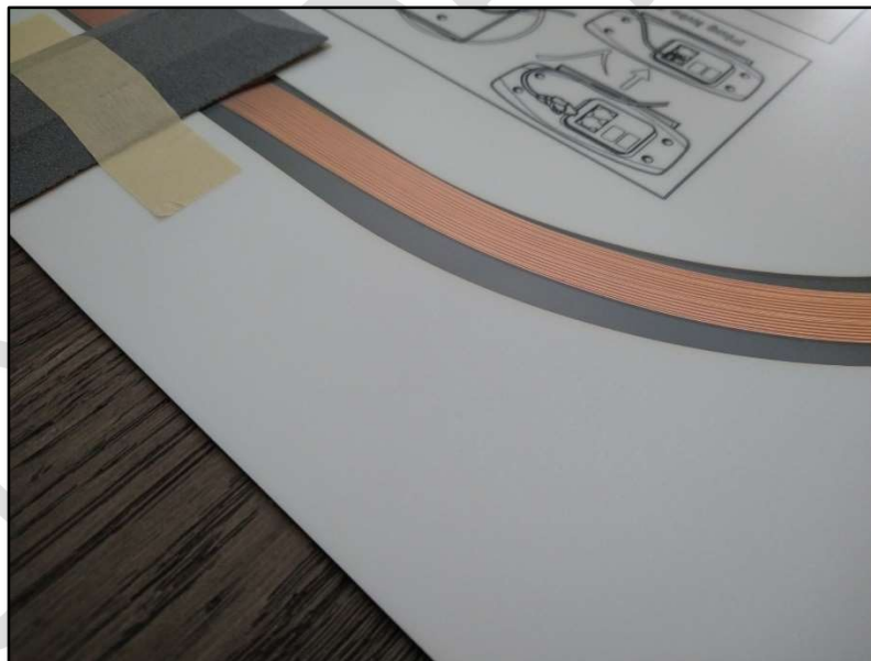
Figure 4. Closeup of production prototype flat spiral coil antenna
