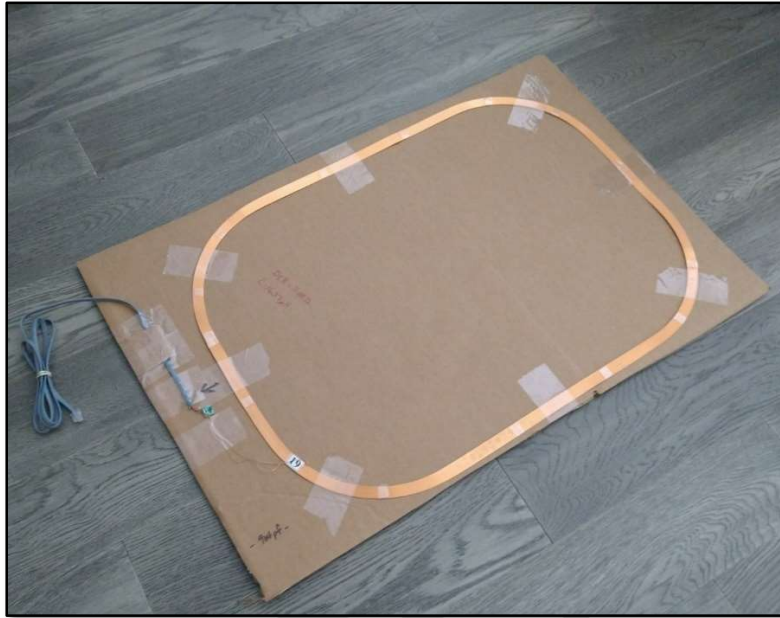
Figure 1. Prototype flat spiral coil antenna
