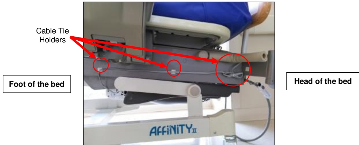
Figure 5. AC Line Power Sensor Cable Routing
