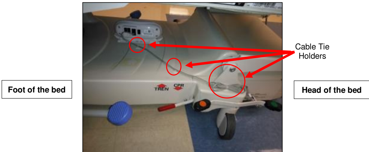
Figure 6. AC Line Power Sensor Cable Routing
