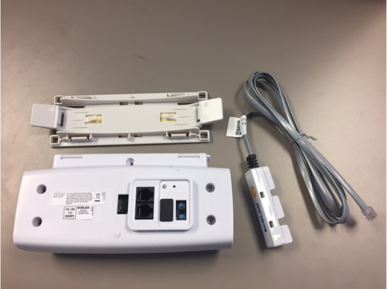
Figure 1. Bed Beacon Installation Components
