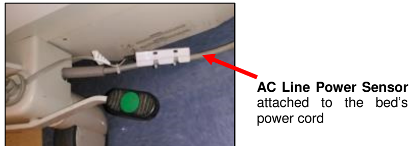
Figure 3. The AC Line Power Sensor Installation Location on the Bed
