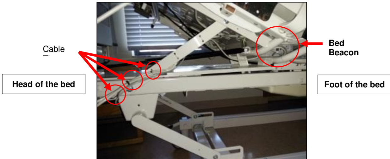
Figure 5. AC Line Power Sensor Cable Routing
