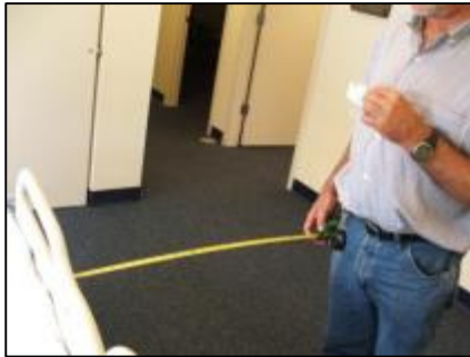
Figure 13. Test Badge Activation Distance from Bed's Handrail Center is 18" (at edge for stretcher installations)
