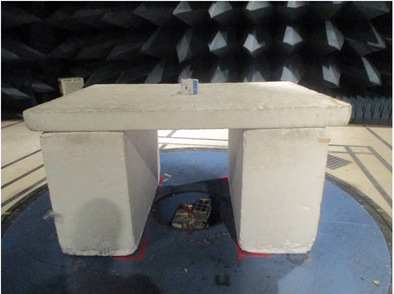
Figure 1: Radiated Emissions – Front View – Below 1 GHz
