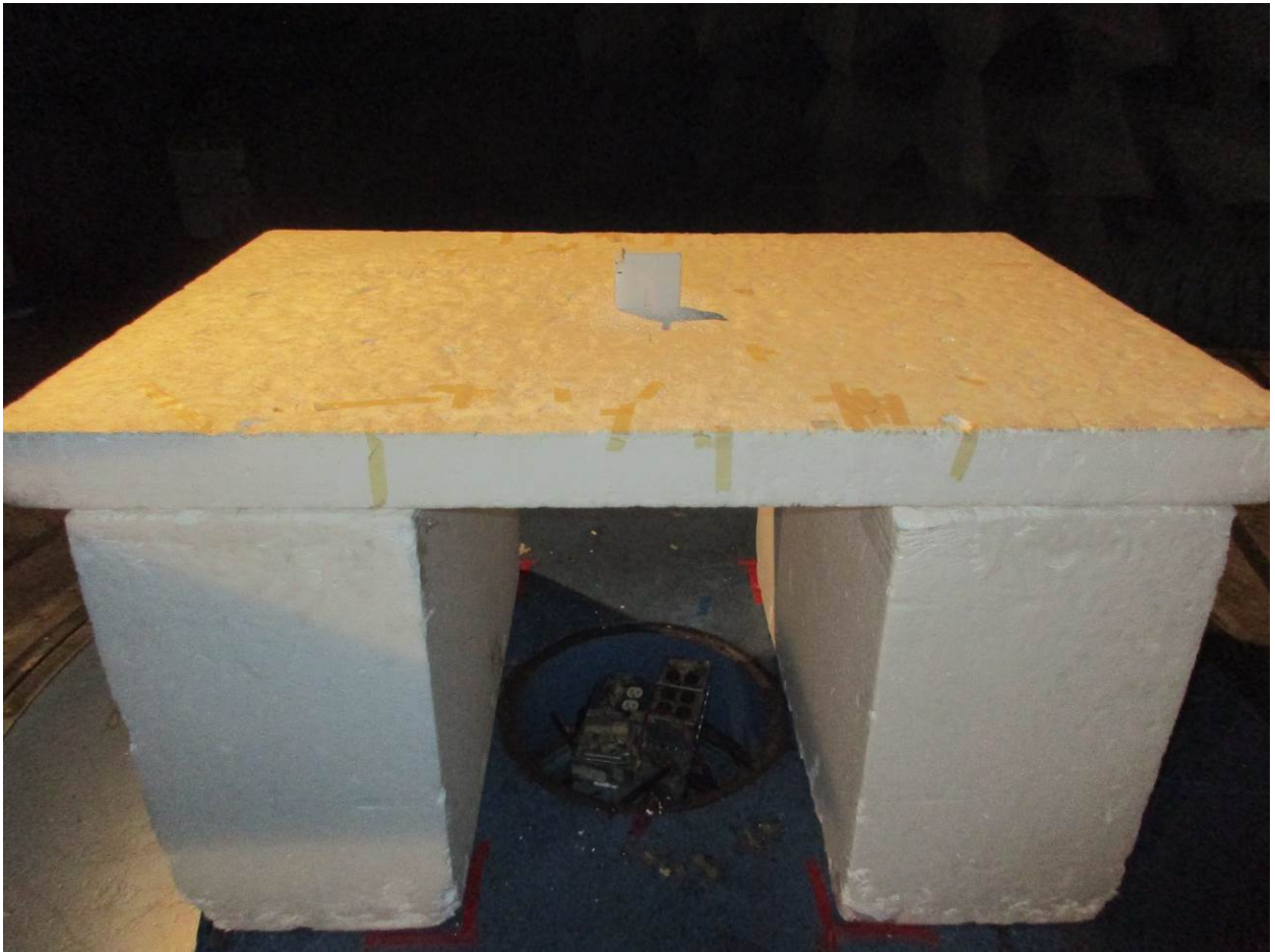
Figure 1: Radiated Emissions – Front View – Below 1 GHz
