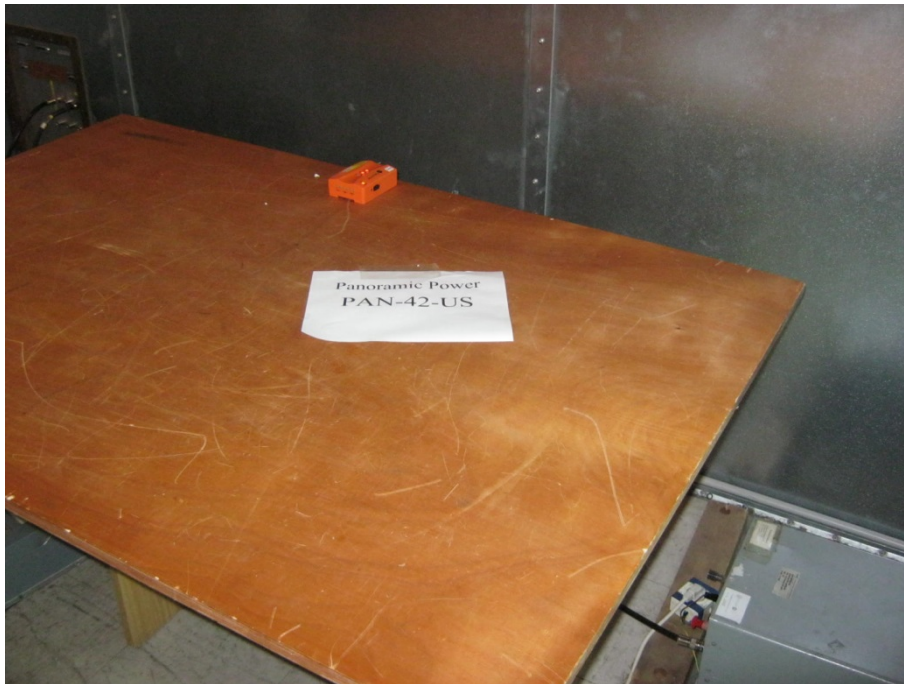
Figure 2. Conducted Emission AC Line Test
