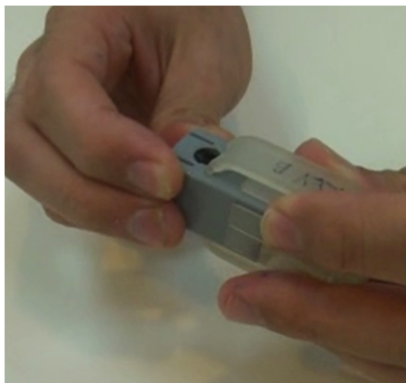
Figure 5. Snap the opener into the sensor holes.
