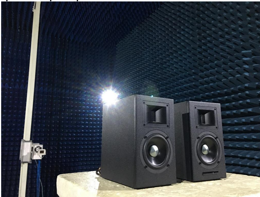
Photograph 4: Set-up for Spurious Emissions for 18 - 26.5GHz
