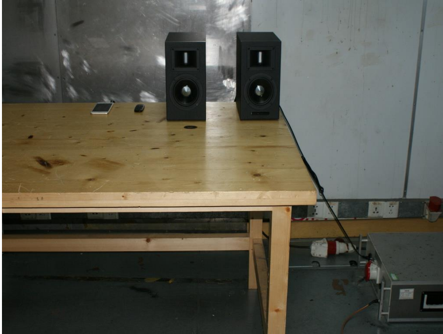
Photograph 5: Set-up for Conducted Emissions
