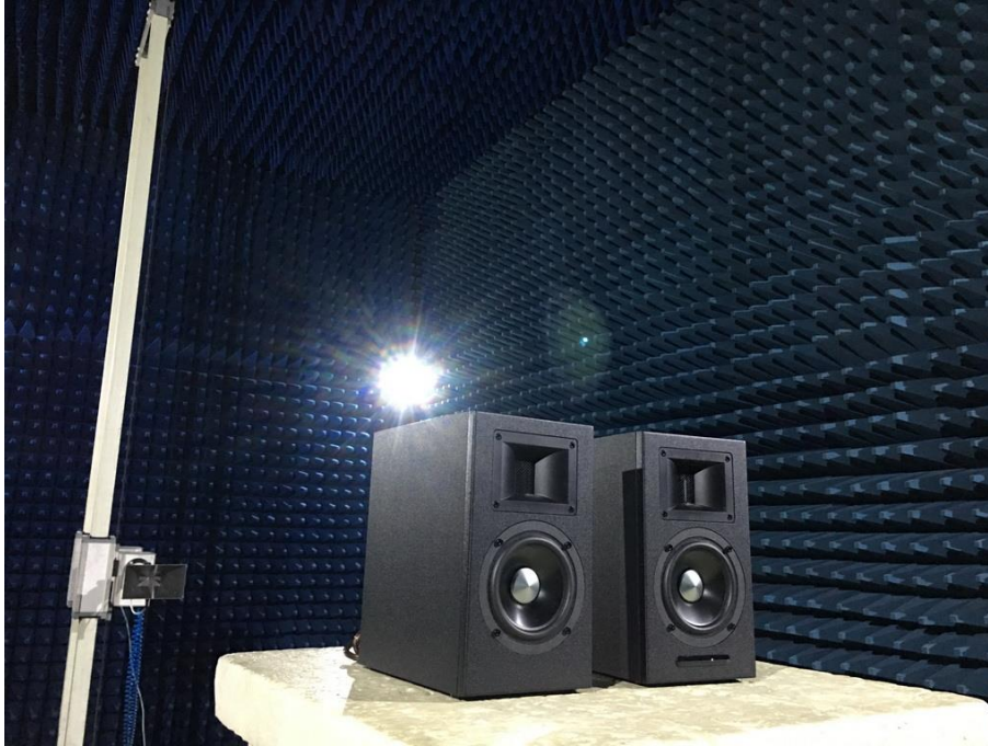
Photograph 4: Set-up for Spurious Emissions for 18 - 26.5GHz
