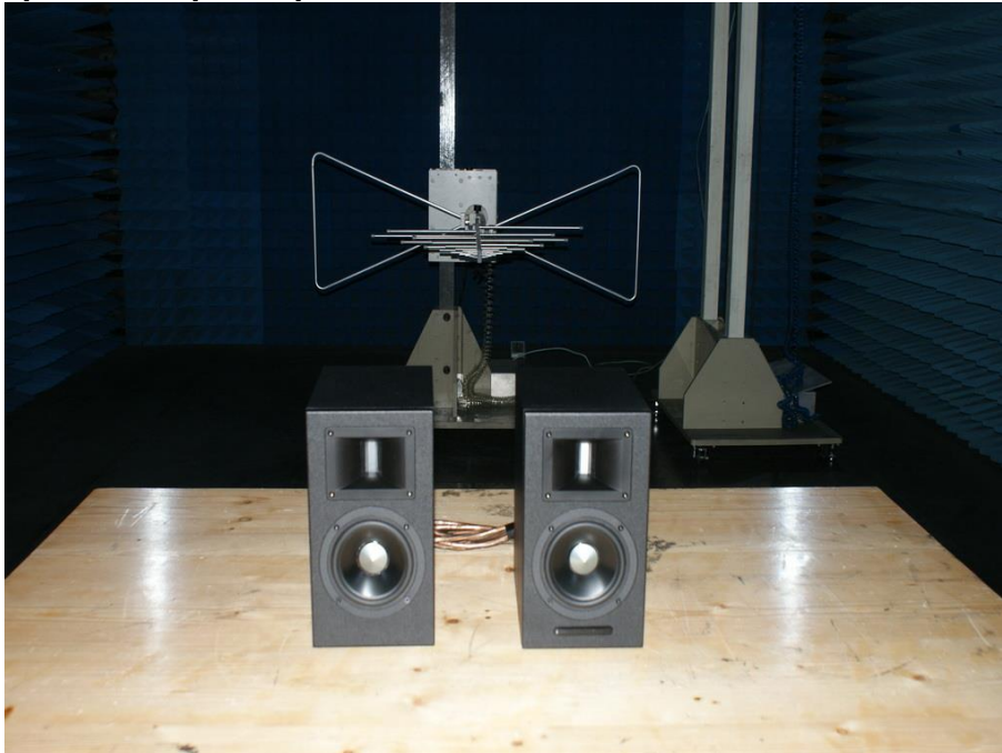
Photograph 2: Set-up for Spurious Emissions for 30 - 1000MHz
