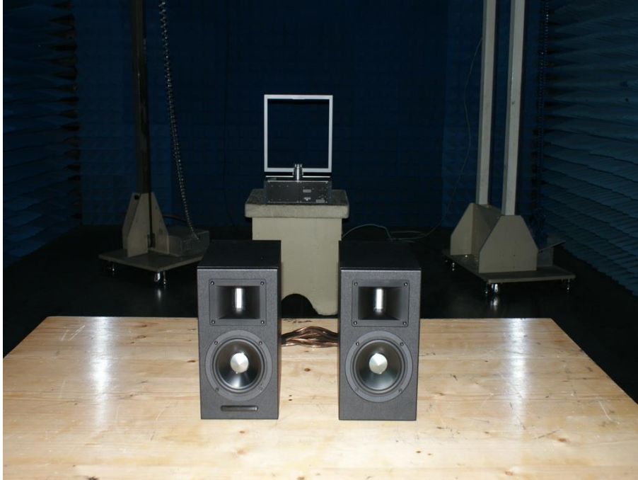
Photograph 2: Set-up for Spurious Emissions for 30 - 1000MHz
