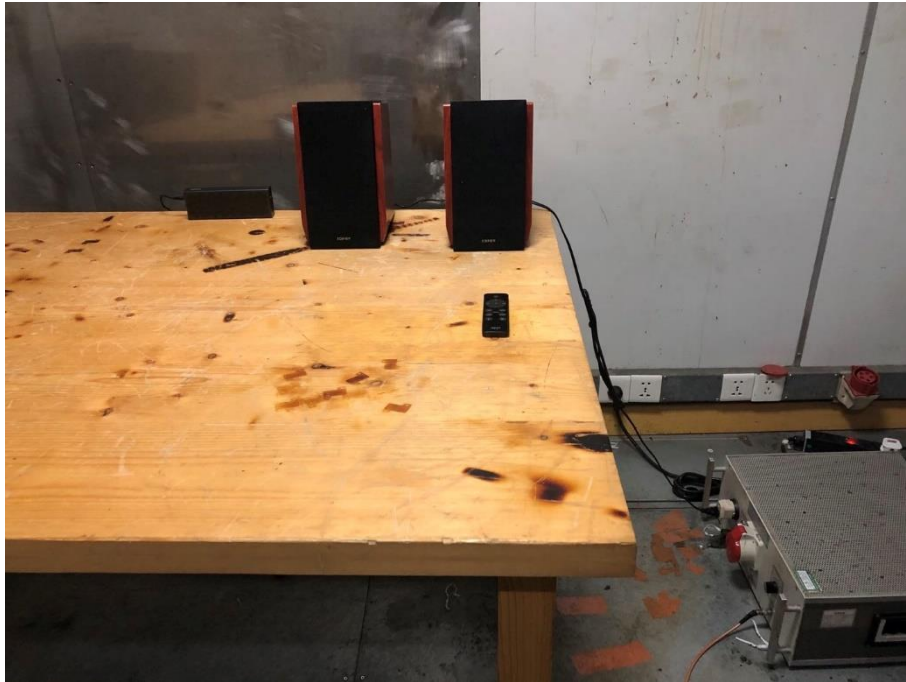
Photograph 3: Set-up for Conducted Emission on AC Mains
