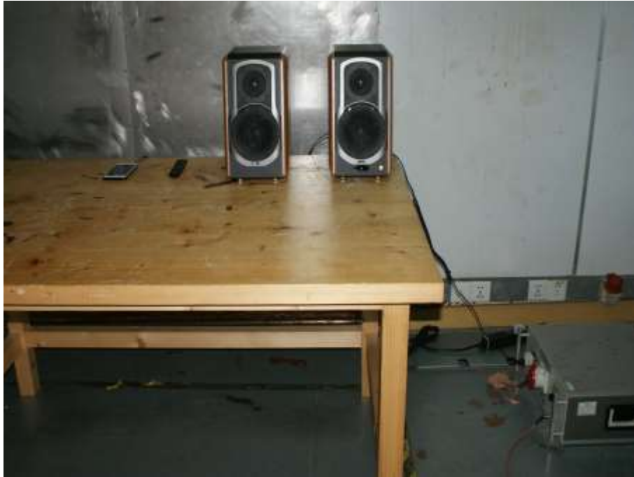
Photograph 1: Set-up for Conducted Emission on AC Mains
