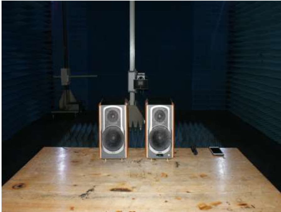
Photograph 4: Set-up for Radiated Spurious Emission, below 1GHz
