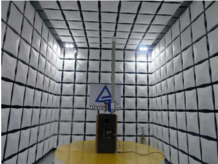
Photograph 5: Set-up for Radiated Spurious Emission, above 1GHz
