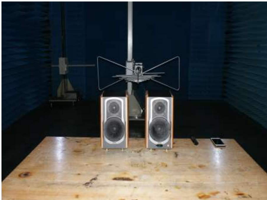
Photograph 2: Set-up for Radiated Emission, below 1GHz
