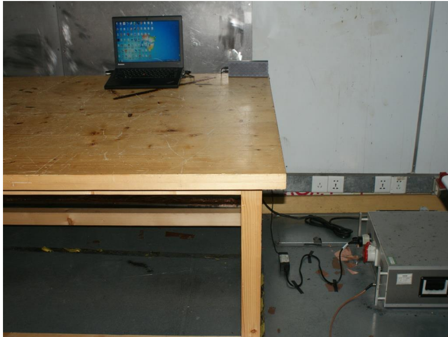
Photograph 3: Set-up for Conducted Emission on AC Mains
