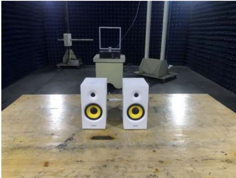
Photograph 2: Set-up for Radiated Spurious Emission, 9KHz - 30MHz
