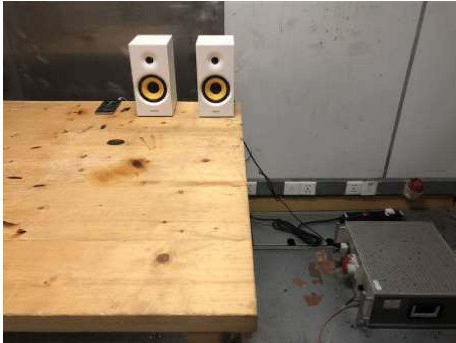
Photograph 1: Set-up for Conducted Emission on AC Mains
