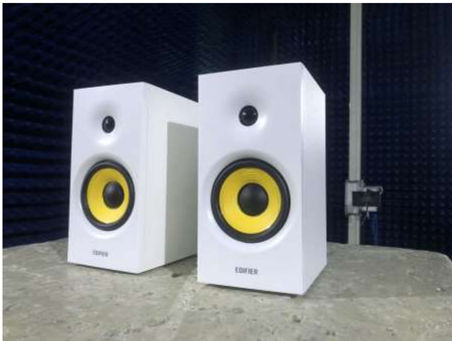
Photograph 4: Set-up for Radiated Spurious Emission, 1GHz - 18GHz
